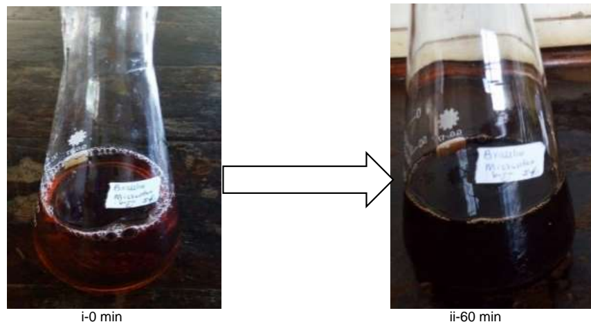
Figure 2. B. micrantha bark extract and AgNO 3 solution on sonication (i) 0 min (ii) 60 min of sonication.
